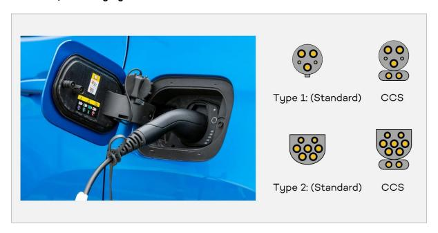
In Europe, the most common type of charging cable is a Type 2, however there are some manufacturers that use a Type 1. Manufacturers will provide the correct one when the vehicle is purchased from new. Charging stations are configured to take either cable, it is the connection at the vehicle that differs.
