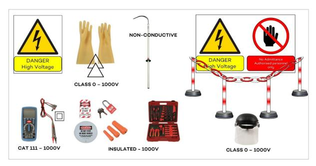
As a minimum, all automotive repair/service business that engage with Hybrid or Electric vehicles should have the appropriate PPE and Tooling:
