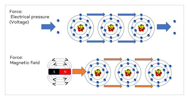
The valance electrons will move from one atom to another if we apply a force. The amount of force needed to make this happen is relative to the bonding strength between the electrons and the nucleus.
