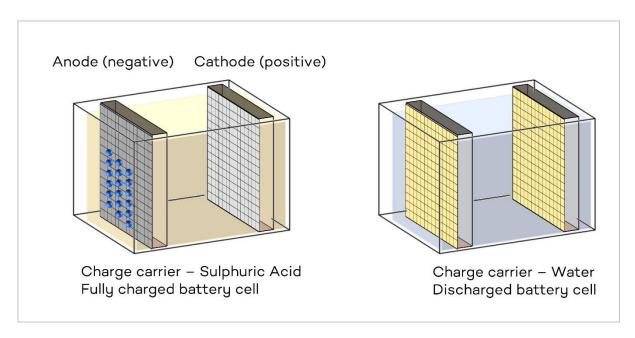
The porous Lead negative plate (Anode) absorbs the charged Oxygen atoms from the electrolyte to become Lead Oxide. As this chemical change occurs the negative plate builds up an excess of charged electrons.
