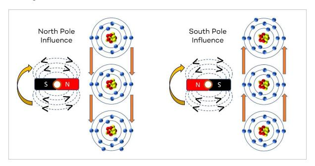
What makes a magnet different to other materials? Remember that materials are made up of atoms, the electrons within those atoms move around constantly and randomly. A magnet on the other hand has special properties, the electrons are held stationery and line up in a uniform pattern. This property creates an invisible force of energy around the magnet referred to as a magnetic field (Lines of flux). The field has two opposing yet equal poles, a North and a South.
