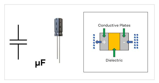
A Capacitor is an electrical component that stores electrical energy, a bit like a battery. Unlike a battery, no chemical process takes place, so it is unable to produce energy. It can discharge the stored energy in a fraction of the time it takes a battery. Capacitors will store energy at a level that matches the voltage supplied to it.
