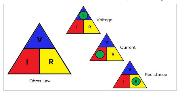
Amperage and Resistance. If we change one of these variables it will affect the other two. In the same respect, if we know what two of the variables are we can calculate the third. This makes electricity predictable!
