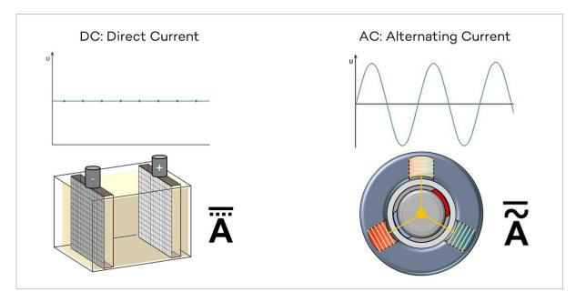
When a conductive path is created between the negative and positive plates of a battery, the electrons will move! This process will continue until the plates have an equal potential (electrical pressure).
