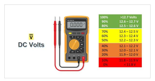
The State of Charge of a battery is the measurement of the amount of energy available from the battery. The measurement is often represented as a percentage.
